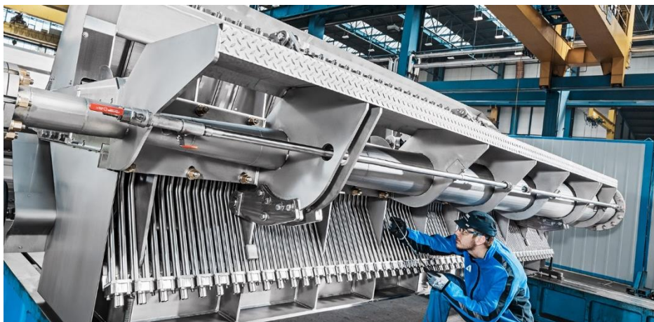
ANDRITZ PrimeFlow AT headbox – superior flow uniformity with unique, accelerating trapezoidal flow tube
