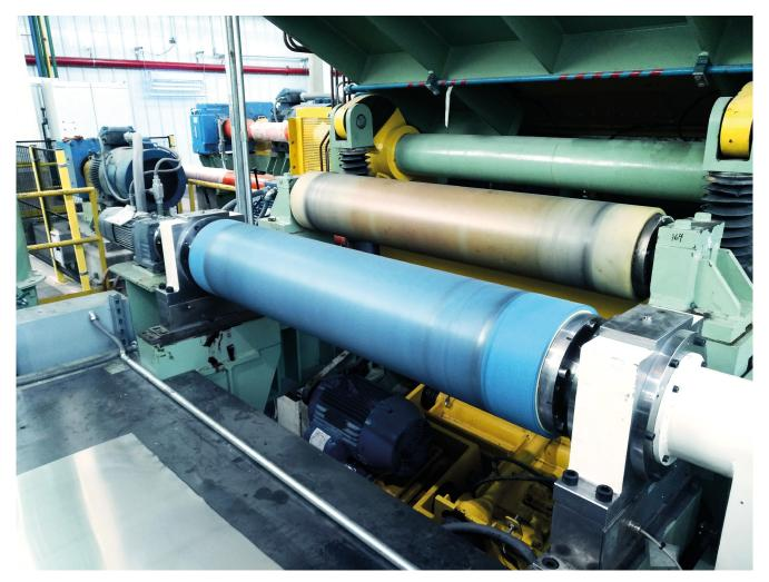
Example for a rubber covered shapemeter roll in a strip processing line
