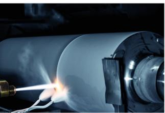
Tungsten carbide plating on a shapemeter roll
