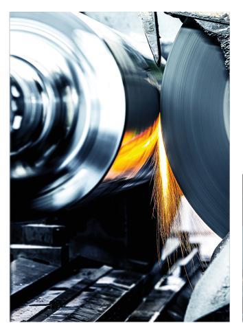
Grinding of a shapemeter roll
