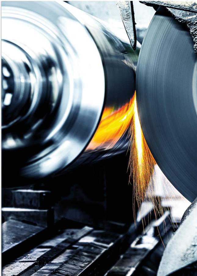
Grinding of a shapemeter roll
