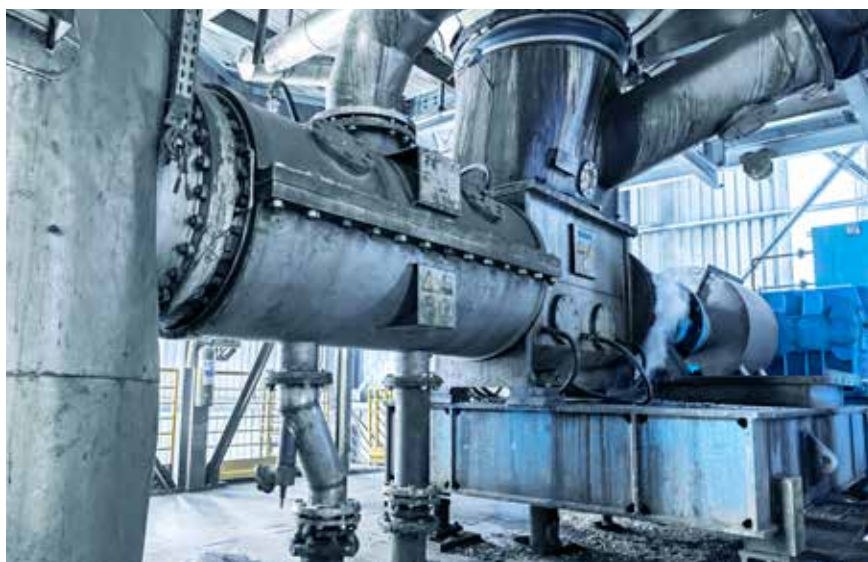
20" plug screw feeder in operation at Guararapes - line 2
