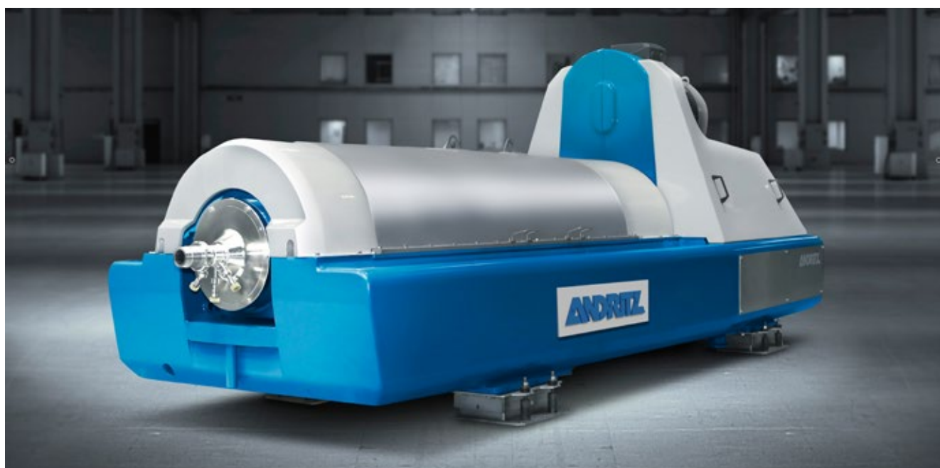
ANDRITZ decanter centrifuges A are a modular series for unrivalled dewatering
