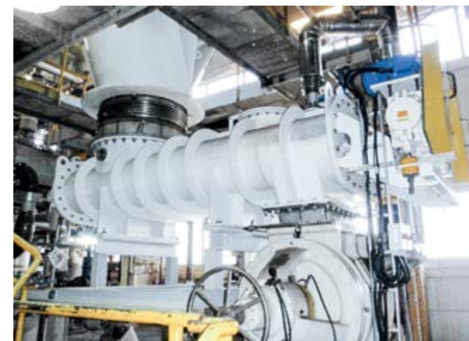
Diamondback™ chip bin bottom and chip metering screw provide uniform chip flow.
