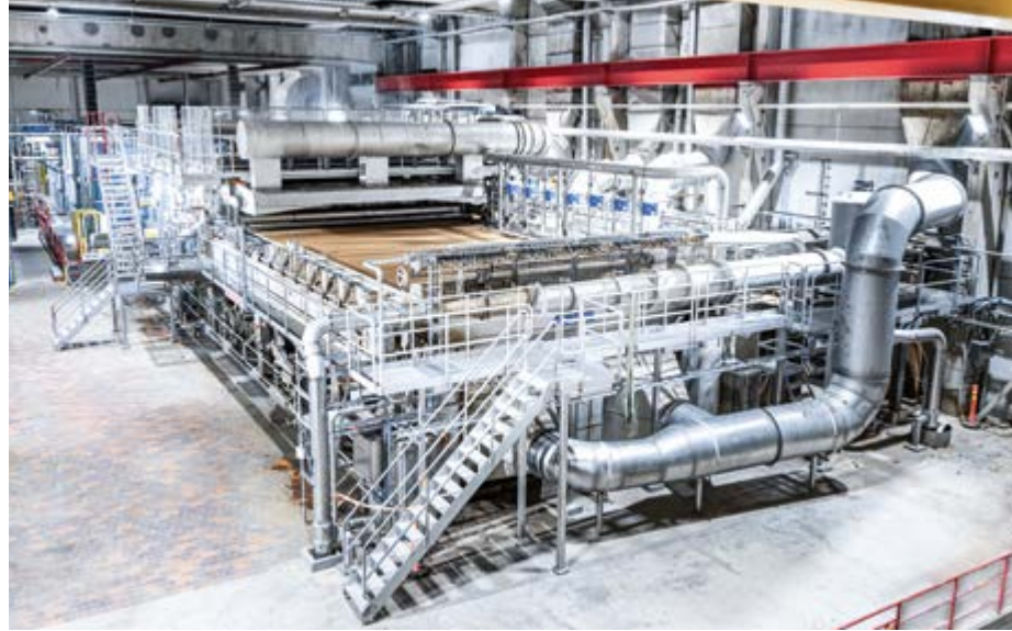
The upgrade project included a rebuild of the complete pulp drying line.
