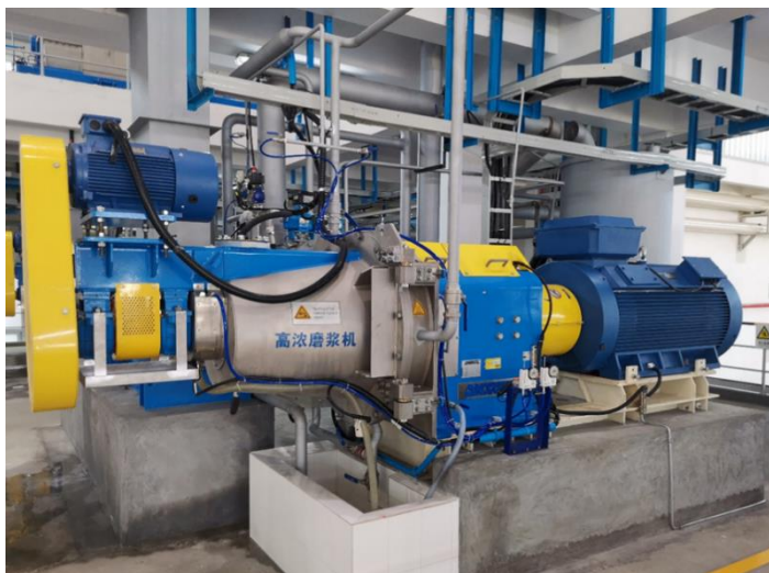
ANDRITZ HC refiner at Vinda Personal Care's Yangjiang mill
