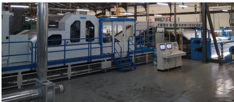
ANDRITZ batt forming line in operation at Romatex, Cape Town
