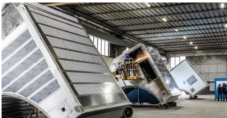
Workshop view: PrimeDry Hood technology to improve heat-transfer efficiency and optimize drying.
