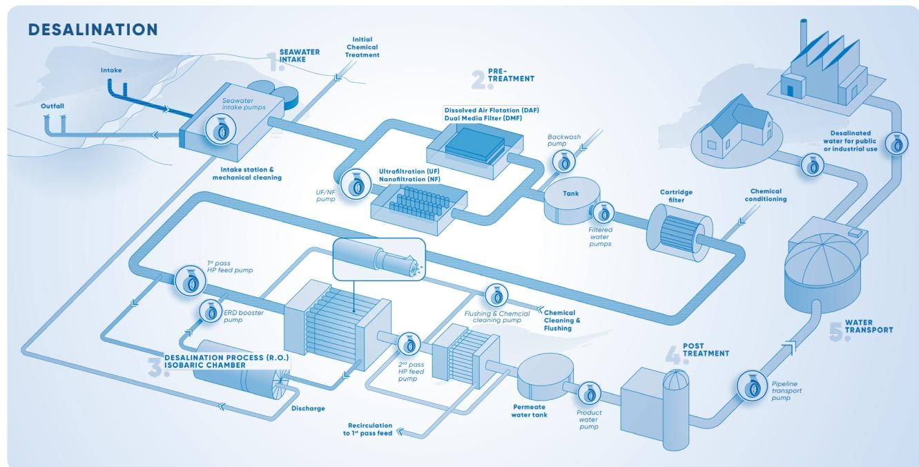
Apart from these pump solutions, ANDRITZ provides a comprehensive range of pumps designed specifically for desalination applications.
