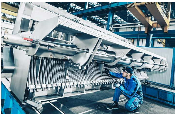
PrimeFlow AT (Accelerating Tube) headbox at the ANDRITZ workshop in Graz, Austria
