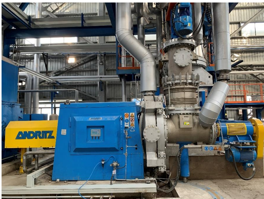
ANDRITZ 1CP refiner at the heart of the pressurized refining system
