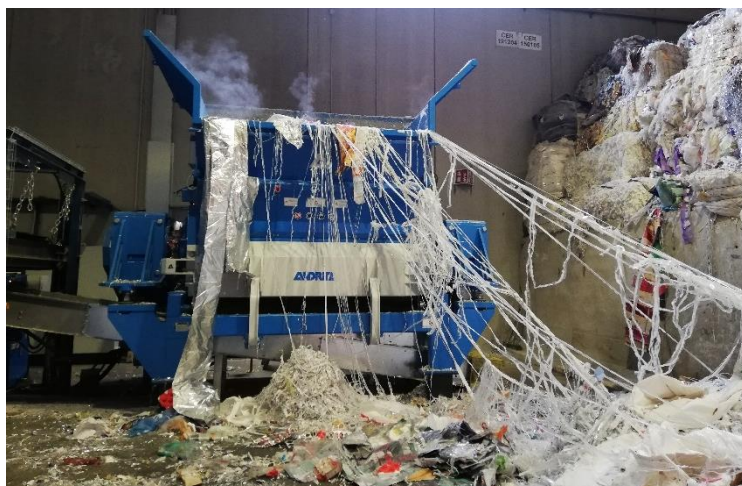
The new ADuro P-3000F shredder for RDF production
