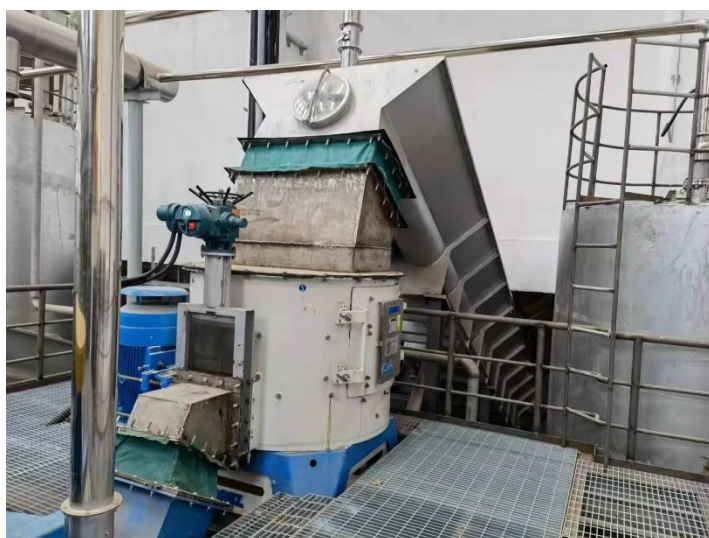
ADuro QZ1600BIO shredder for kitchen waste treatment
