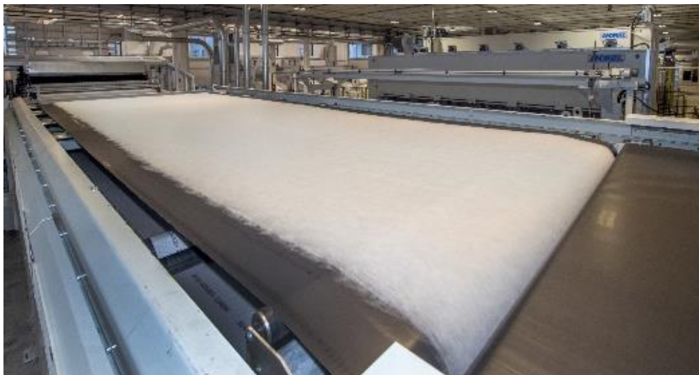
ANDRITZ eXcelle crosslapper in operation
