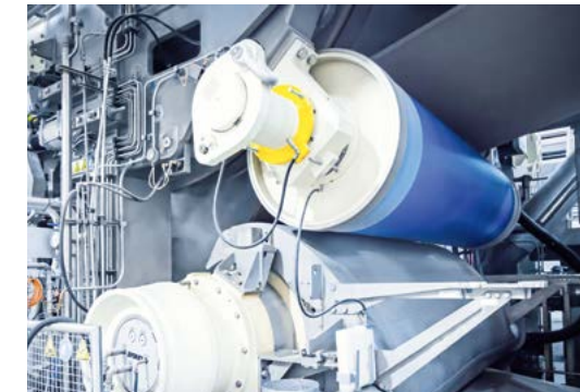
The combination of a 16 ft. PrimeDry Steel Yankee and the latest PrimePress XT Evo shoe press technology enables a high drying capacity and achieves remarkable cost savings and operational flexibility as well as improved product quality.
