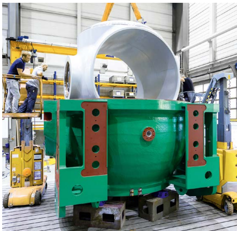
Assembly of valve rotor into MIV housing
