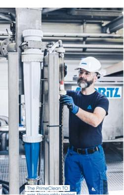
at ANDRITT's Stock Preparation Pilot Plant The PrimeClean TO is the newest addition to the ANDRITZ family of low consistency hydro-cyclone cleaners. It is ideally suited for recycled fiber and approach flow applications with feed consistencies up to 3%.
