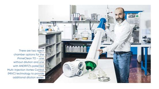
The new PrimeClean TO is the latest innovation in cleaners from ANDRITZ. The "TO" designation comes from the fact that it combines two cleaning stages in one unit (two-in-one). Thanks to its innovative reject chamber design, the PrimeClean TO is ideal for removing sand and small particle debris from approach flow stock and recycled fiber processing lines at higher feed consistencies. The first systems have been sold and start-up is planned for early next year.
