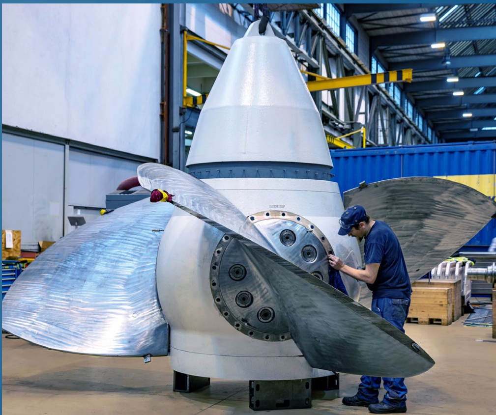
Manufacture of the new Kaplan impellers and factory overhaul of the large turbine components will be carried out at ANDRITZ's manufacturing facility in Ravensburg, Germany.
