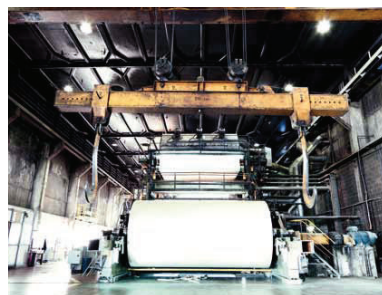
▲ The surface properties of the folded boxboard are significantly improved, thanks to the new top ply. Operators can now reduce the grammage of this ply, resulting in lower raw material costs.
