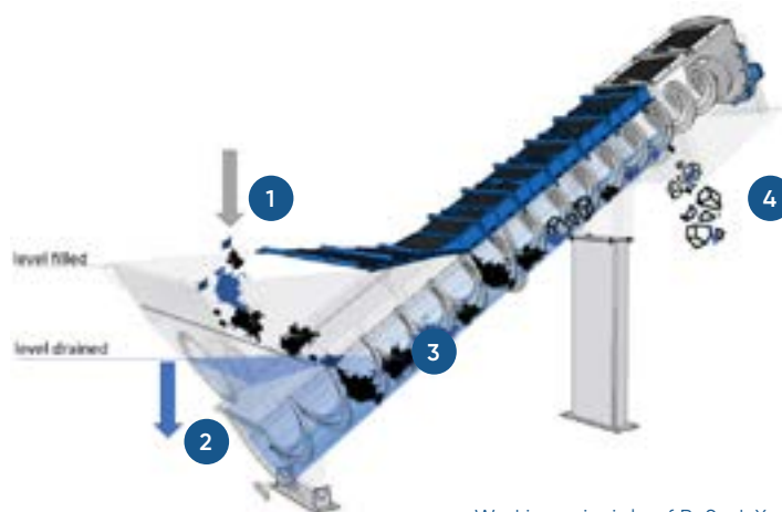
Working principle of ReSed-X
