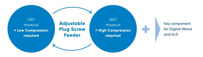
Online adjustable compression setpoint with closed control loop.
