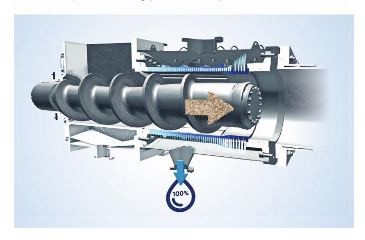
With the Adjustable Plug Screw Feeder ("Adjustable PSF"), ANDRITZ offers a patented world innovation that transforms a static system into a dynamic one. The new cylindrical plug screw can now be moved back and forth in its axis by up to 10 cm. Thanks to the specially designed conical nose, the size of the gap between the screw and the spool piece can be varied to increase or decrease compression during ongoing production.
