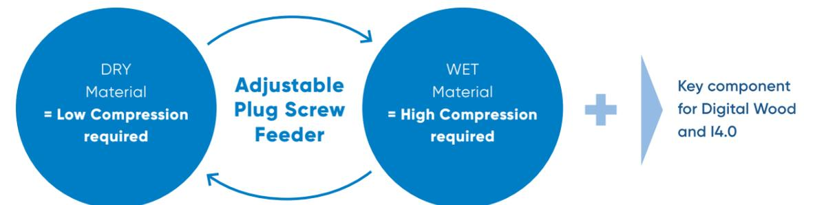
Online adjustable compression setpoint with closed control loop.
