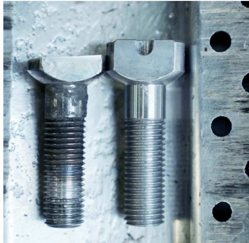
Fixation bolt with new (right) and worn wear indicator.
