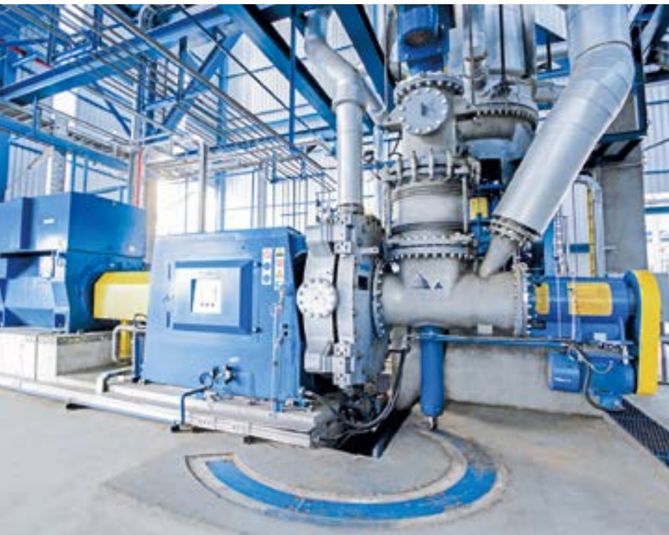
ANDRITZ S2070 high-consistency refiner.
