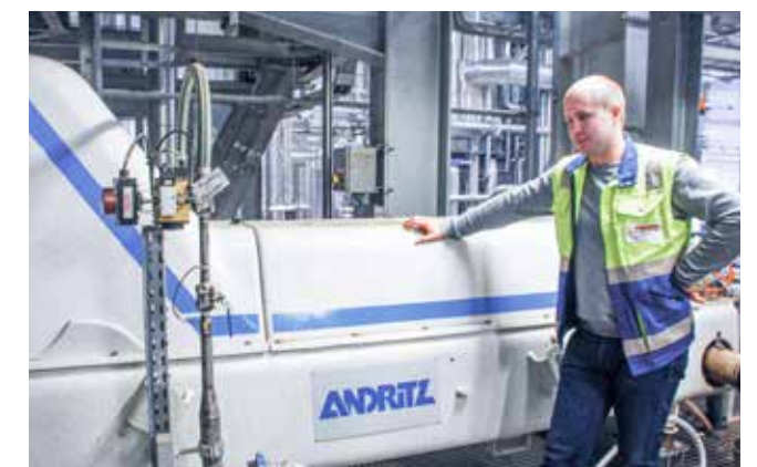
The ANDRITZ decanter removes finest particles from the recycled wash water.
