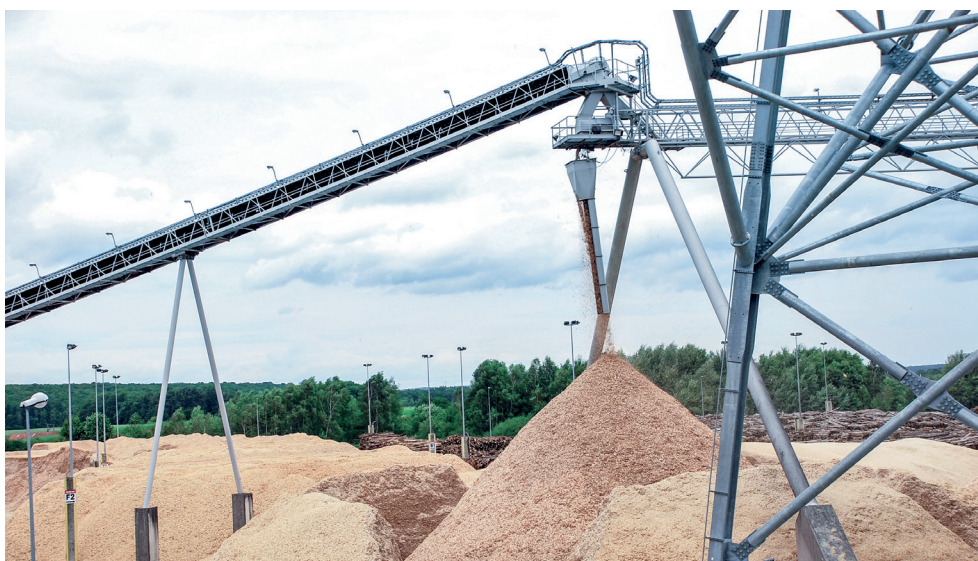
The six-day capacity chip handling and storage system from ANDRITZ includes chip conveying, chip receiving pocket, chip storage, reclaiming and screening. A huge woodyard at Norske Skog next door provides essential security for Pavatex's steady production flow.
