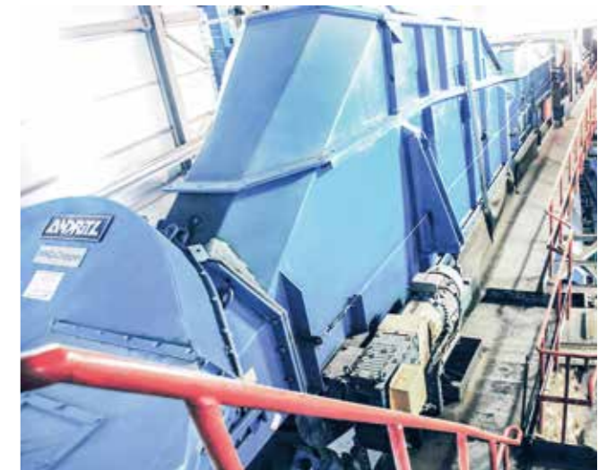
The ANDRITZ HHQ Disc Chipper, horizontally fed, equipped with 10 knives for a capacity of 300 m 3 sob/h.
