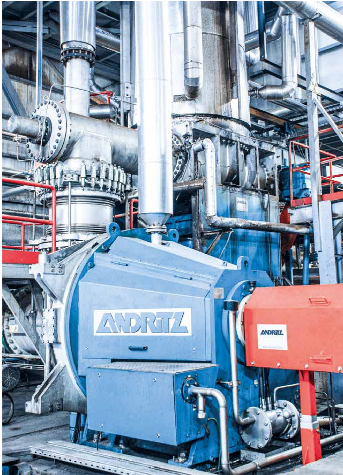
ANDRITZ S 2070 refiner: chips in - high-quality fibers out
