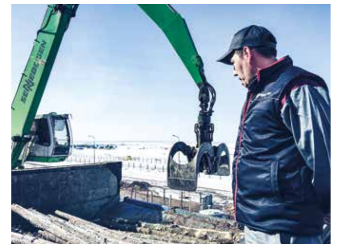
Logs are discharged into a bin, where they begin their journey to the debarking plant. Pine and spruce are the choice for HDF. Birch and aspen are the species for MDF.
