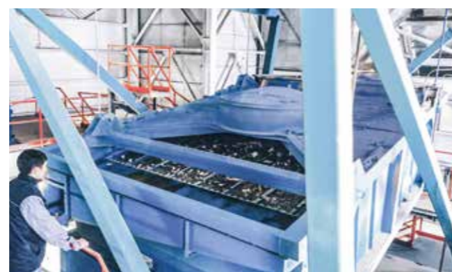
ANDRITZ screens remove undesirable, matchstick-sized wood after chipping.
