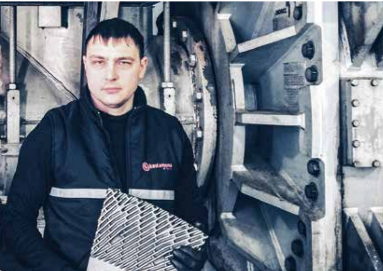
Plates for Line 1's pressurized refiner are specially designed for pine and spruce for HDF, and birch and aspen for MDF. This refiner produces high-quality fiber for the Siempelkamp press line.
