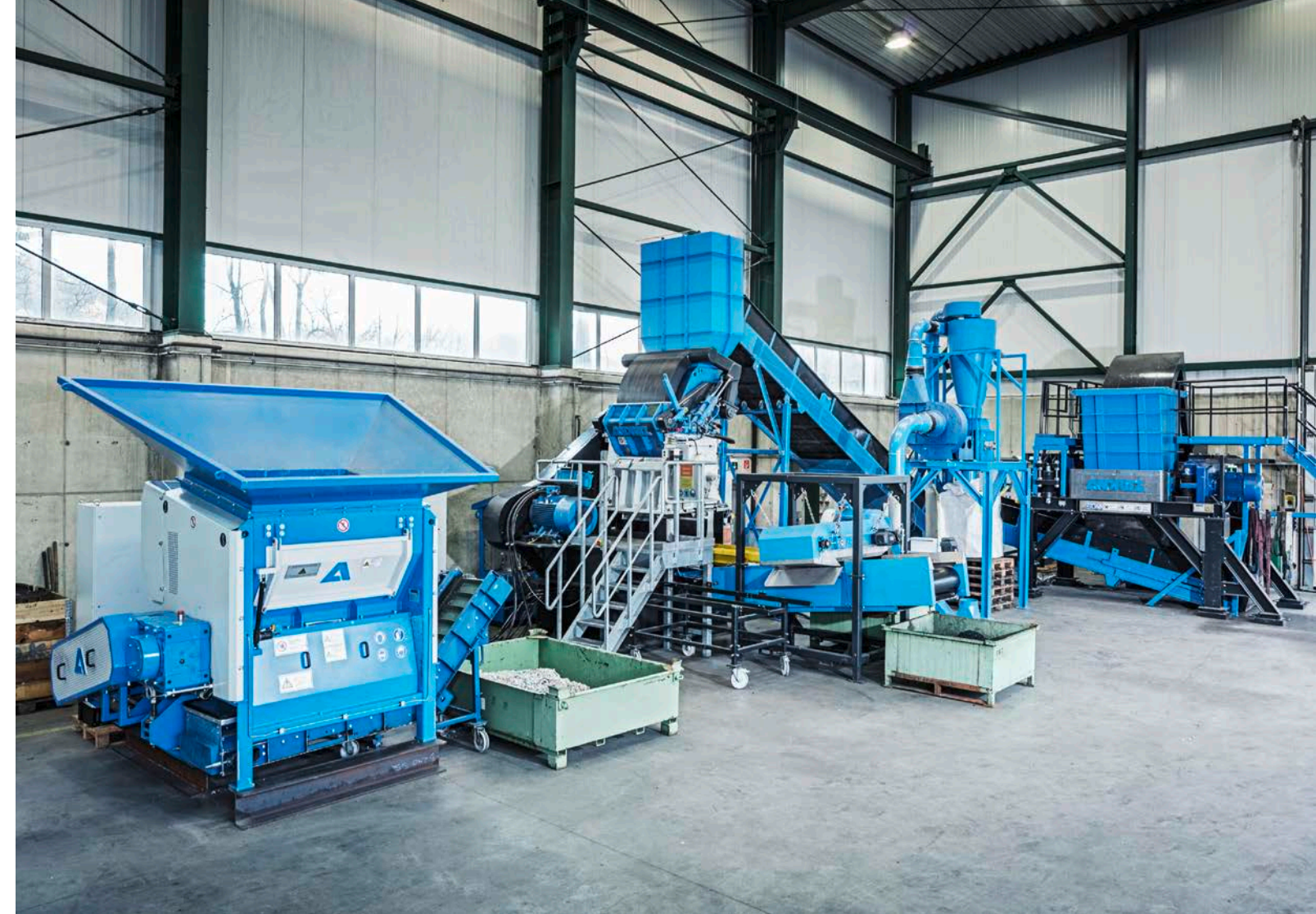
ADuro shredders for primary and secondary shredding as well as for fine granulation and dismantling
