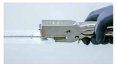
4.2 The end of a stainless steel zipper is normally secured with staples.
