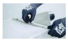
Secure the bag with the holding plate. The bag should be pulled up as far as the fabric allows or until the rope is touching the bottom of the clamp.
