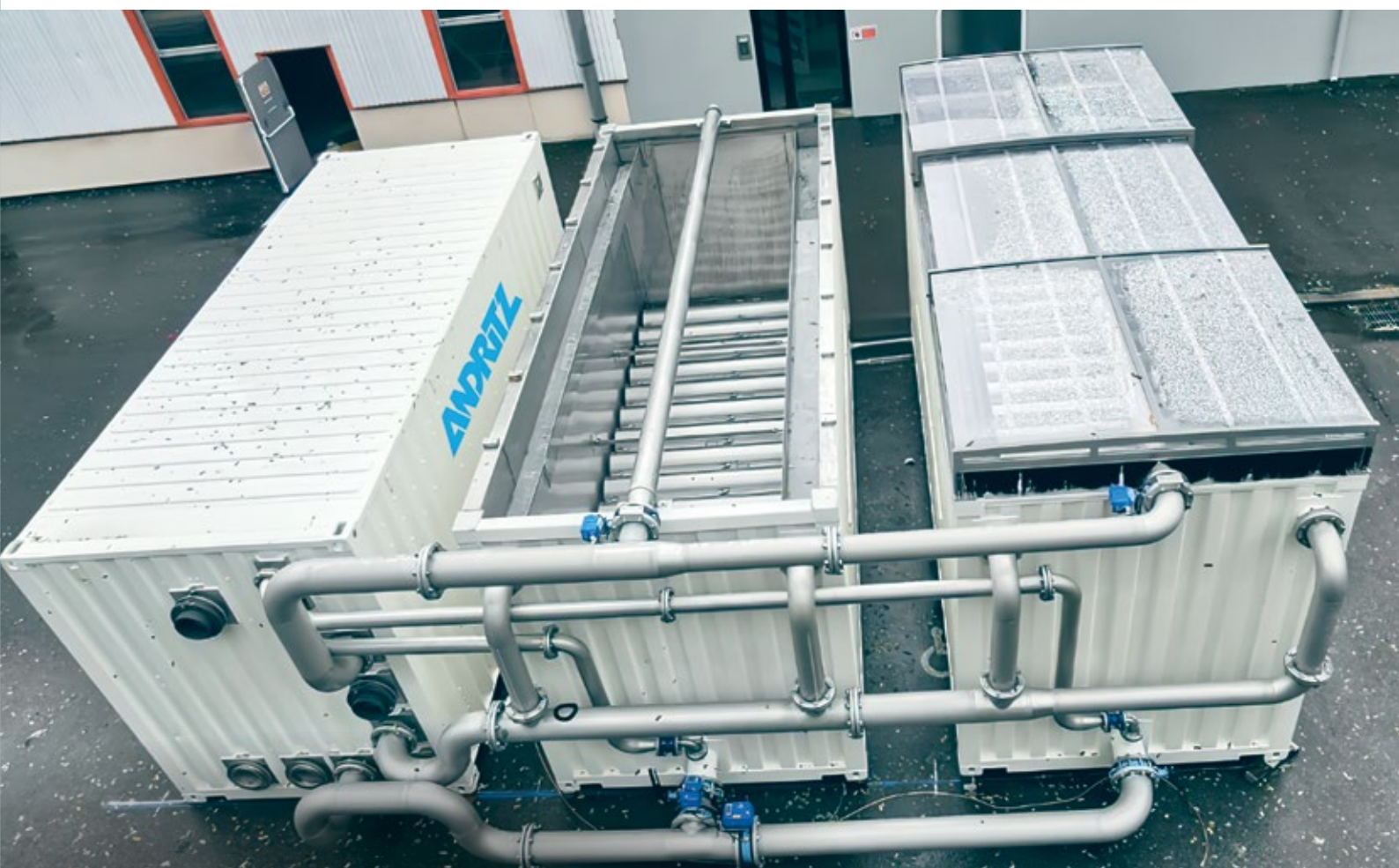
ANDRITZ Mobile Filtration Unit (AMFU) made up containers (process and filtration)
