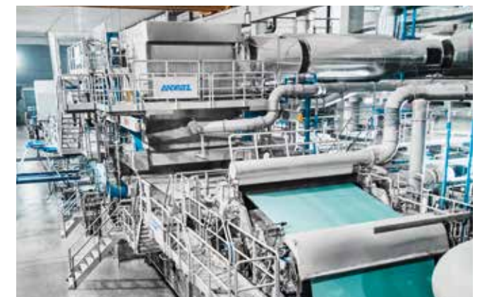
PrimeLineCOMPACT tissue machine with a design speed of 1900 m/min
