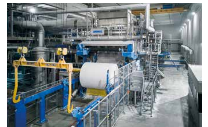
PrimeReel comes with nip-load compensation
