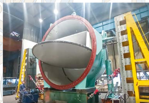
PIV during FAT (Factory Acceptance Test) at ANDRITZ' workshop in Hungary
