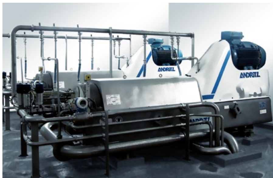
Decanter centrifuge for removal of liquid phase from vegetables
