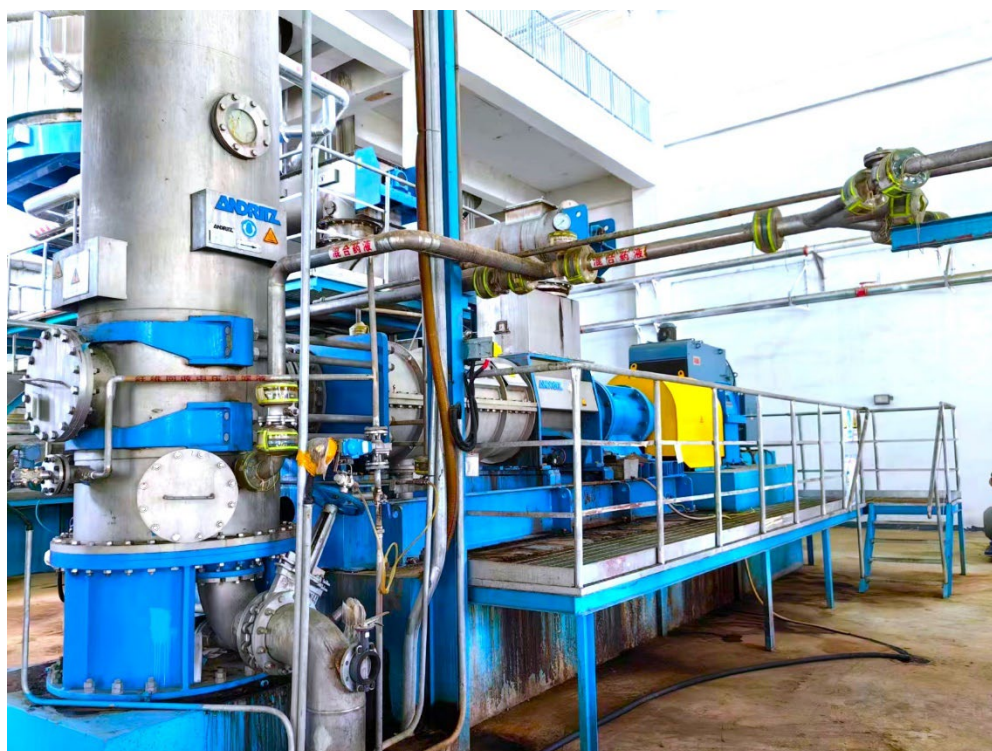
ANDRITZ PrimeMSD Impressafiner and vertical Impregnator running in Taiding mill
