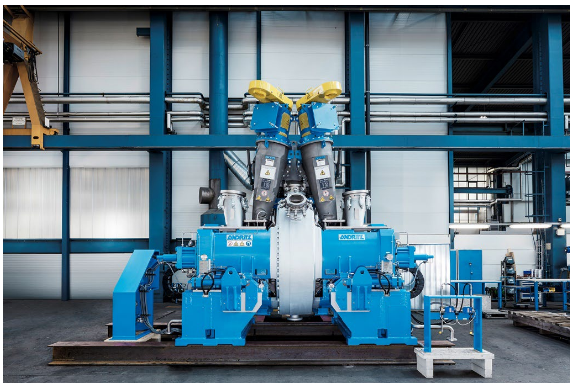
High-capacity and high-performance refining with the ANDRITZ TX68 refiner
