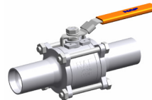
NAF 888652/62 DN 15-65, PN 10-40 NAF 888352/62 DN 80-100, PN10-16 Face-to-face length acc. to DIN 3202-F1 and ISO 5752 serie 1 Flanges
