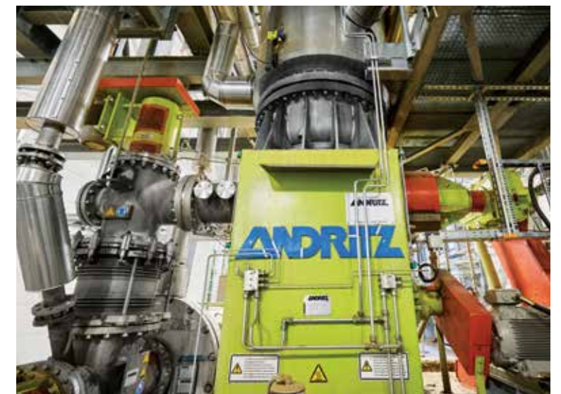
Very even feeding of the material to the refiner with the well-proven ANDRITZ C-feeder
