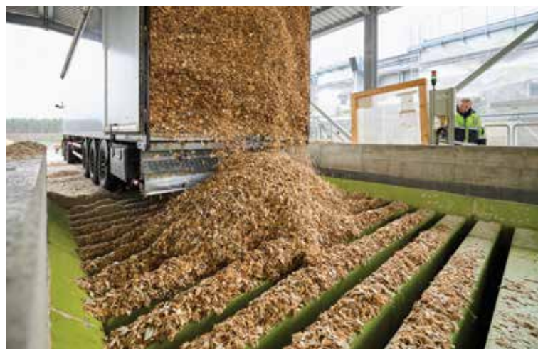
Tilting floor for constant and high throughput of the bulk material.
