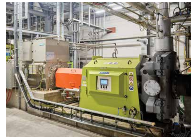
High-consistency (HC) refiner ensuring a constant refining gap that is essential to obtain high fiber quality.
