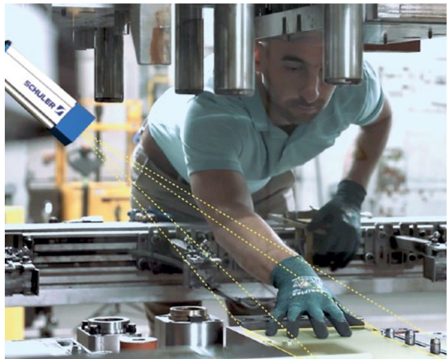
Metris Visual Die Protection detects foreign objects or other sources of danger in real time and stops the line before any damage occurs.
