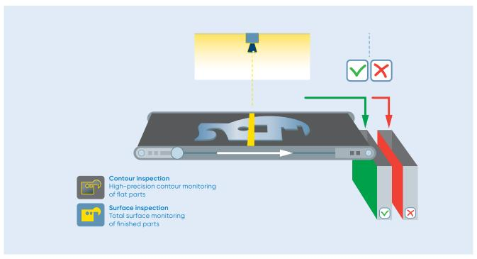
Visual Quality Inspection is an adaptable add-on that provides security for your quality control – camera-based and smart.
