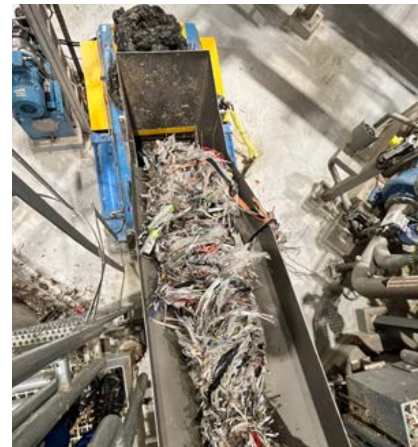
Online rag processing: The pulper rags are pulled out of the pulper, cut, and shredded fully automatically.
