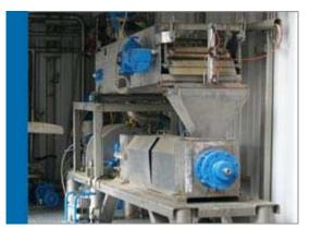
Gravity table and sludge screw press in the mobile test unit
