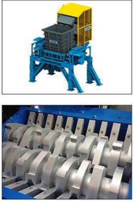
Cutting unit of the ANDRITZ Rotary Shear UC
