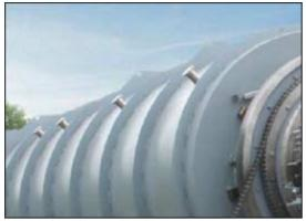
Pyrolysis reactor: The plastic turns into a hot gas that is cooled and becomes pyrolysis gas or oil, and the remaining metals can be recycled in the metals industry.
