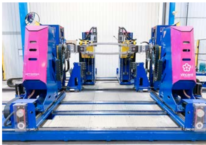
Peterborough, Canada – Coil spreading process for Carillon hydropower project
