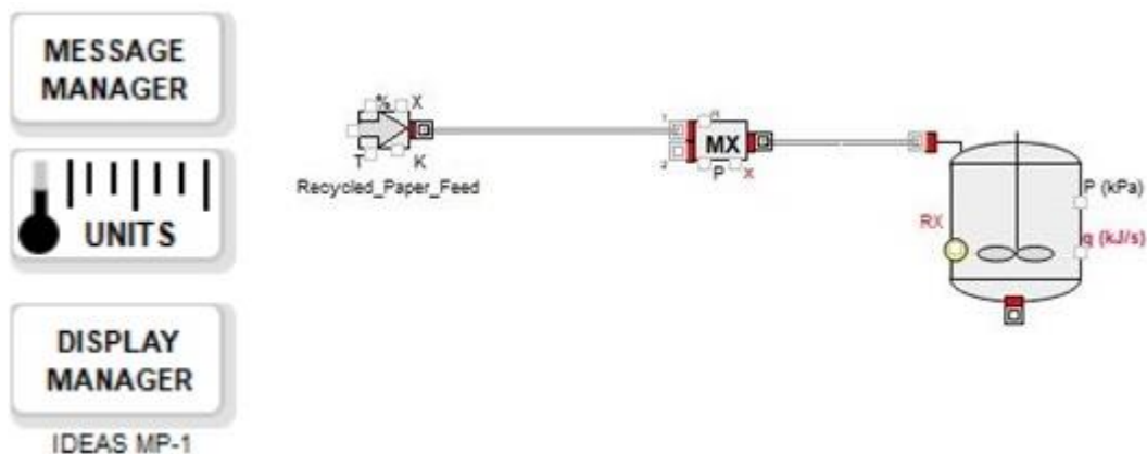
Figure 22: Placing and Connecting of Mixer and Reactor RX
