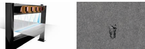
High Angle Reflection Web Inspection
