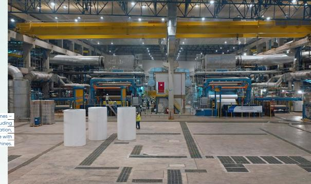
Four complete tissue production lines from stock preparation to the reel, including fabrics and rolls, pumps, digitalization, services, and maintenance with PrimeLineTM W 2000 tissue machines.
