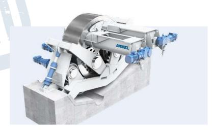
To go along with the HQ-Press, ANDRITZ has also devised a dedicated steam injection system for increasing the temperature of the bark before pressing it. Silventoinen says, "By increasing the temperature of the bark bark, for example, to 45-50°C, the viscosity of the water in the bark will be lower and we can obtain a better pressing result. Our steam injection solution can also be used to ensure that the bark always reaches a minimum of 15°C before pressing."
