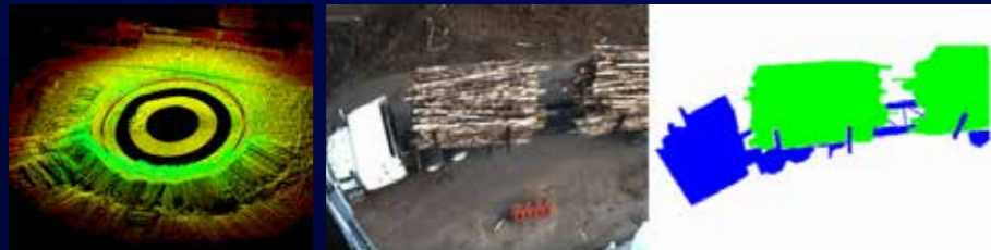
Real-time 3D scan of the crane environment. Machine vision object detection and segmentation.
