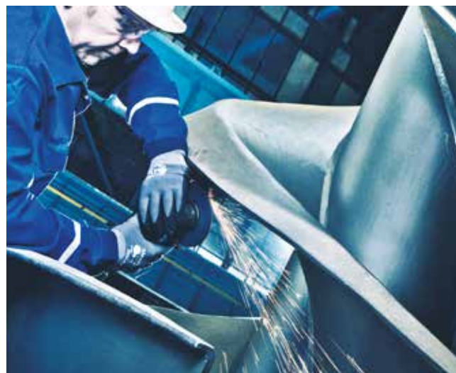
Pulper rotor repair of all kinds in the Levice service center
