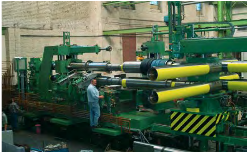
▲ Slitting shear for hot-rolled strip with automatic tool change turnstile
