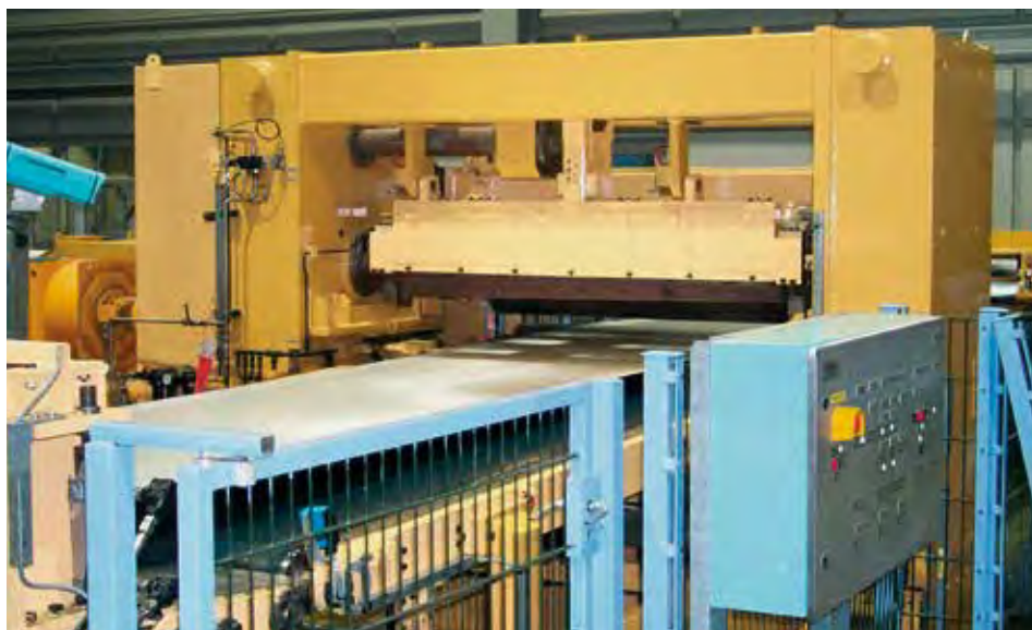
▲ Rotating shear for fast scrap cutting in inspection lines
