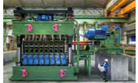
▲ Leveler for plates with a thickness up to 60 mm
